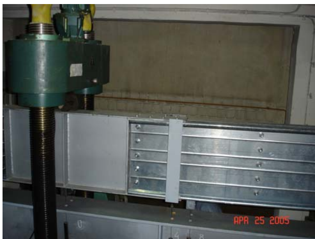
Fig. 8 The GN beam during the test
