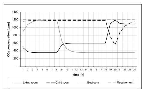
Figure 7. Carbon dioxide concentration runs for alternative no. 3
