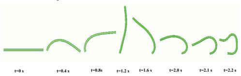
Figure 6: Nonlinear dynamic response of rod subjected to an applied rotation.
