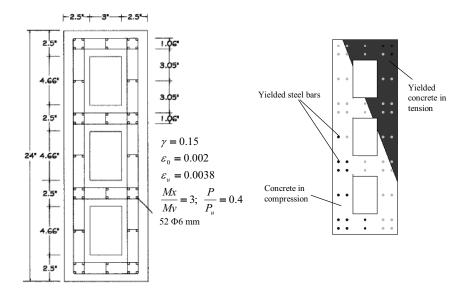
Figure 6. Rectangular RC Hollow Pillar. (a) Cross Sectional Properties and Reinforcement Arrangement; (b) Plastic status at  $\varepsilon_u$ =0.004.
