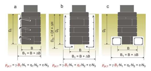
Figure 3. Consolidation procedures of continuous footings: a. one side covering, b. two sides covering, c. introducing of adjacent foundations
