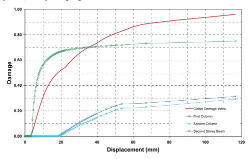
Figure 10 - Evolution of the global damage and the member damage indexes at the second floor
