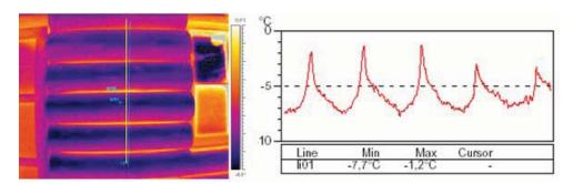
Figure 4. Thermo camera outputs – outside view
