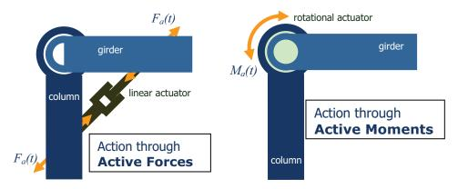
Fig.3 Structural Active Hinges development, SAH [29]
