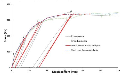
Figure 8 - Comparison of the experimental results with results obtained by using the frame analysis with the proposed platic-damage model, and a finite element model.
