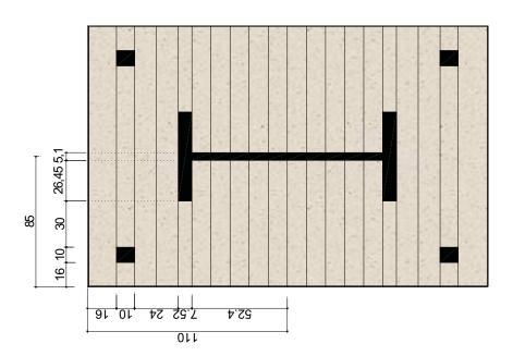
Figure 4. The assimilated cross section
