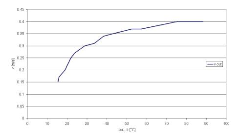
Figure 9. The dependency of the air velocity coming out of the gas space heater on the difference of air temperatures coming out of the gas space heater  $t_{out}$  and the interior air temperature  $t_i$
