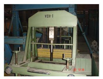
Figure 1. The electodynamic vibrator built by professor Varlam from the Bridges Laboratory of the Faculty of Civil Engineering in Iasi.
