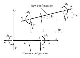
Figure 3. Transfer of the current nodal forces to the new configuration
