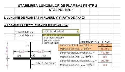
Figure 2. Introducing the supports at the column ends
