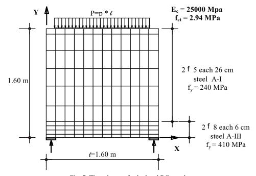
Fig. 7. The schema of calculated RC panel
