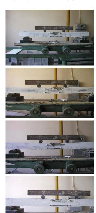
Fig. 7 Failure mode and crack pattern
