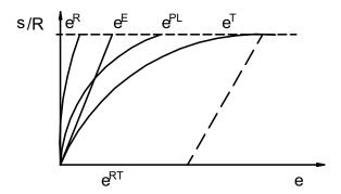
Fig. 1. Stress-strain relationship for concrete.
