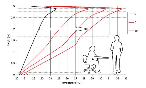
Figure 6. The vertical air temperature difference; warming-up
