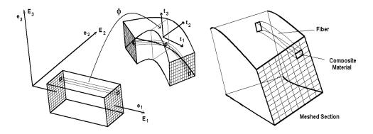
Figure 1: Kinematics of beams and grid of quadrilaterals in each section.
