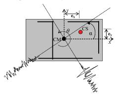
Figure 3. Floor plan and ground motion directivity
