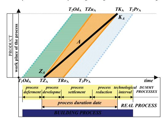
Picture 1. In time-spatial diagram presented behaviour of the process *A* and to it pertaining dummy processes: deferment, technological interval, development, settlement and reduction of the process
