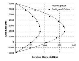
Figure 5. Example 3. Biaxial Interaction Curves.
