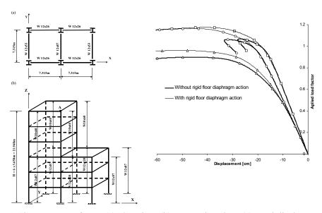
Fig. 4. Six-story space frame: (a) plan view; (b) perspective view; (c) Load-displacement curves at *Y* dirrection for node *A*
