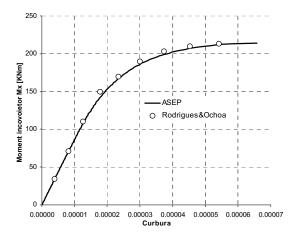
Figure 7 (a) M-N- $\Phi$  Diagrams in X direction
