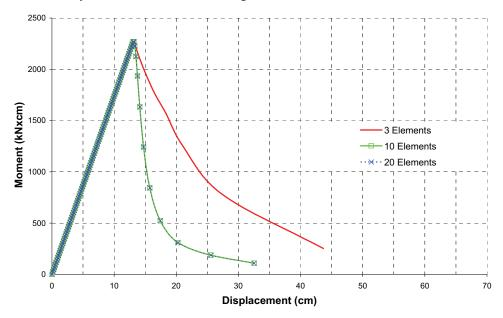
Figure 5 – Moment on the column base versus displacement at the left upper corner.
