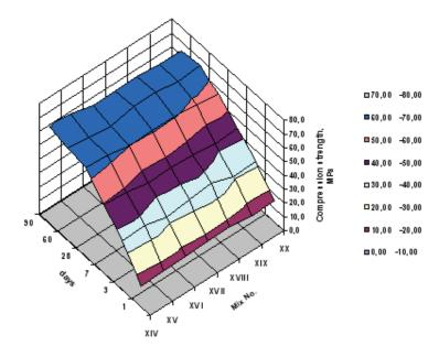
Figure 8. Compressive strength gain with time (11)
