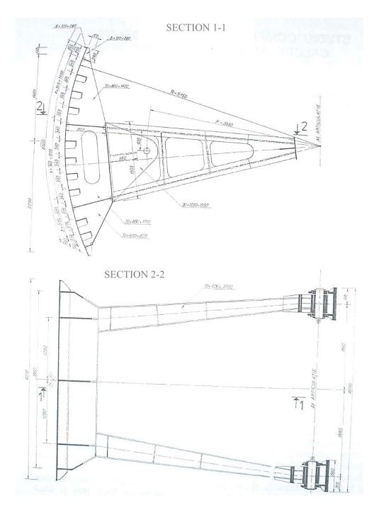
Figure 1. The structure of analized radial gate
