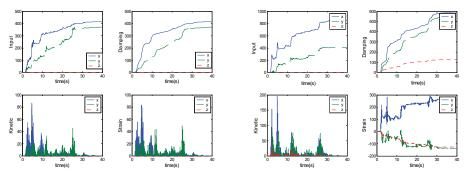
Figure 14. Total energies,  $e_x=e_y=0$ ,  $60^{\circ}$  directivity (kNm, kNmrad<sup>2</sup>)
