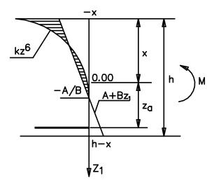
Fig. 5. Self-stress in reinforced concrete beam with crack.
