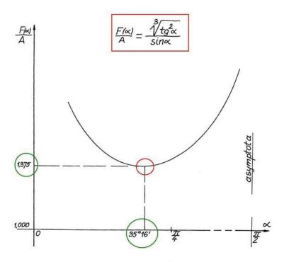
Fig. 3. Solution of question of simple scalar optimization
