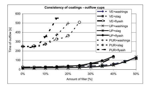
Figure 2. Consistency of polymer coatings in fresh state
