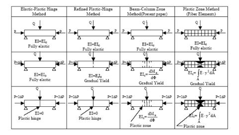
Fig.1 Concept of spread of plasticity for various advanced analysis methods
