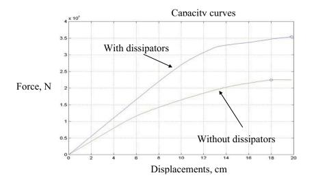
Figure 5: Capacity curves.
