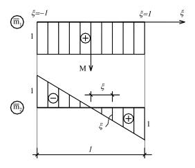
Figure 3. Bending moment diagrams  $\overline{m}_1$  and  $\overline{m}_2$
