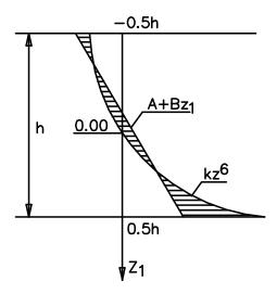
Fig. 3. Self-stress in concrete beam.
