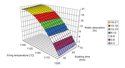
Figure 2. Water absorption - constant pressing pressure 35 MPa
