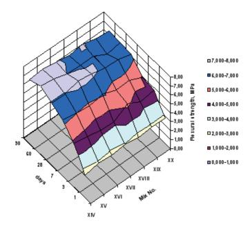
Figure 9. Tensile strength under bending gain with time (12)
