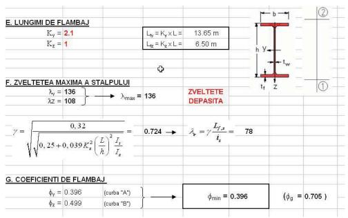
Figure 3. Buckling length and factors
