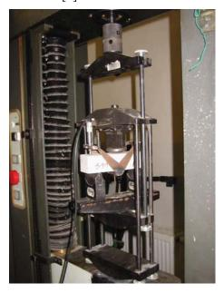
Figure 2. Three-Point-Bending-Test
