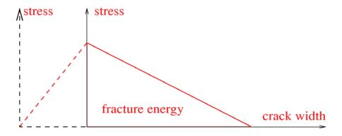
Figure 2. Relation between crack width and stress
