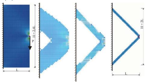
Figure 5. Design domain. ESO solution for R = 5%, 12,5%, and optimal solution for R = 30%.
