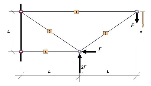
Figure 6: Four-bar plane truss with one loading case
