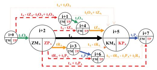
Picture 4. Arc-defined network of the process *A* with description and time evaluation of the arcs (relations and behaviour) and nodes (events) of real process and dummy processes
