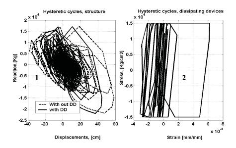
Figure 6: Hysteretic cycles. 1: Structure. 2: Energy dissipating devices.
