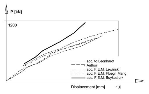
Fig. 9. The relationship between loading and displacement.
