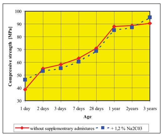
Figure 2. Long-term compressive strength of gypsumfree cements in relation to time
