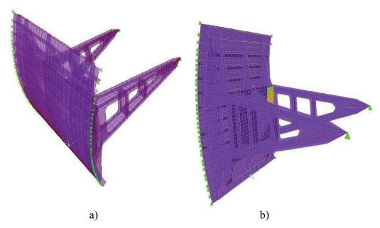
Figure 3. The mesh of the structure; a) view from upstream; b) view from downstream
