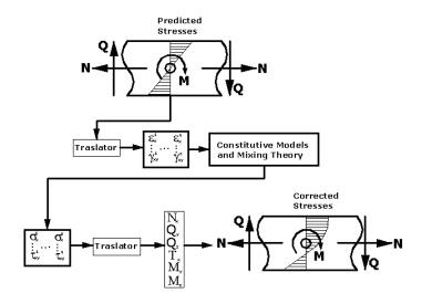
Figure 2: Iterative process at Integration point level in each section.
