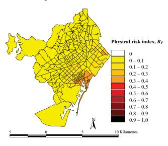
Figure 14: Physical risk index for Barcelona, using the 248 small statistical zones (ZRP)
