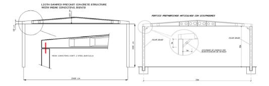
Figure 8: Precast industrial building without and with dissipators.
