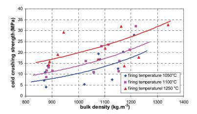
Figure 5. Effect of firing on strength
