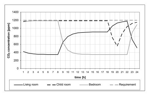
Figure 6. Carbon dioxide concentration runs for alternative no. 2
