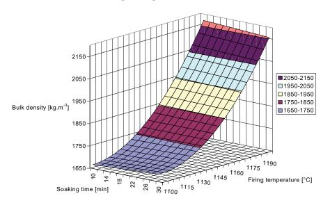
Figure 4. Bulk density – constant pressing pressure 35 MPa
