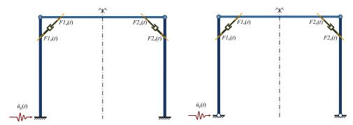
Figure 4. Simple, one span and one level, structures with active control
