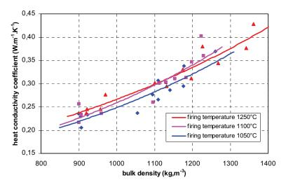
Figure 4. Effect of firing on heat conductivity
