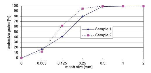
Figure 1. Sieve analysis of washing wastes
