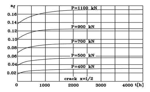
Fig. 3. The dependence of the time and loading levels on the crack width  $a_f$  for x=1/2.
