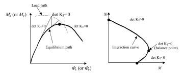
Figure 2. Geometrical representation of the present method.
