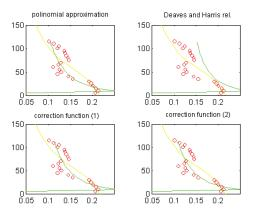
Fig. 4 Graphical representation of the theoretical functions of aproximation of the turbulence intensity (red- values obtained from measurments; yellow- graphical aproximation of the line; green- functions decribed mathematically by the program [5]
