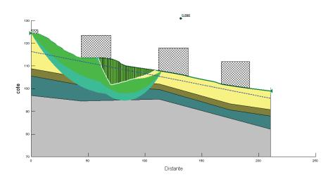
Figure 4. The potential sliding mass and safety factor according to case 4
