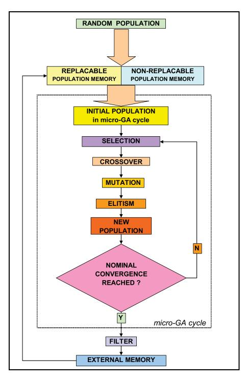
Figure 5: Diagram of micro-GA
