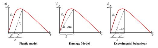
Figure 2 - Loading-unloading behaviour: simulated behaviours and experimental behaviour
