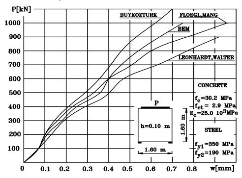
Fig.2. Comparison of calculated load-midspan deflection relations with the test result of panel WT3 [8].
