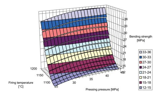
Figure 3. Bending strength – constant soaking time 30 min.
