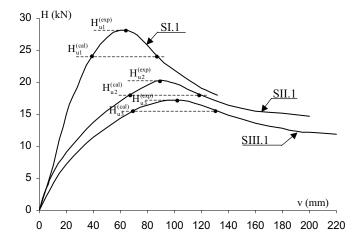
Figure 3. Curves of the monotonic tests
