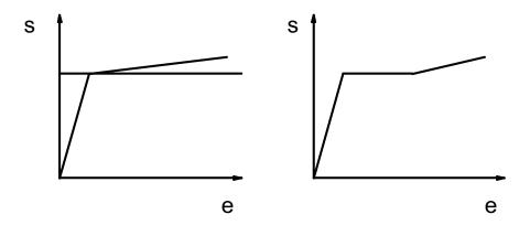
Fig. 2. Stress strain model for steel.
