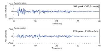
Figure 1. Orthogonal acceleration records, El Centro, May 19, 1940
