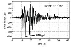
Figure 5. Example of external actions (time-history seismic accelerations)
