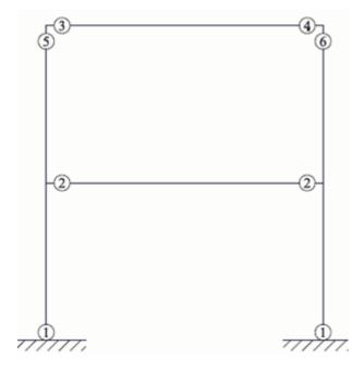
Figure 11 – Sequence of formation of the plastics hinge within the frame.
