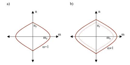
Figure 1 - Yield Surface in m-n space: a) without hardening, b) with hardening.
