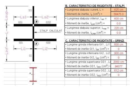
Figure 3. Introduction of stiffness characteristics of adjacent beams and columns
