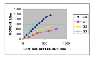
Fig.6. - Midspan moment-curvature for different beams
