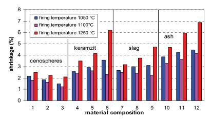
Figure 3. Shrinkage by drying and firing
