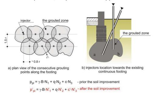
Figure 4. Typical view of a jet grouting technique
