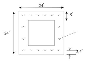
Figure 4. Example 3. Box cross-section with reinforcement arrangement.
