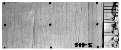
Figure 3. Reference screed mixture with elongation of 1.5% in the direction of the warp
