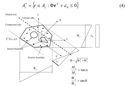
Figure 1. Model of Arbitrary Composite Cross-Section
