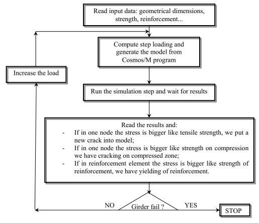
Fig. 3 - Computing algorithm
