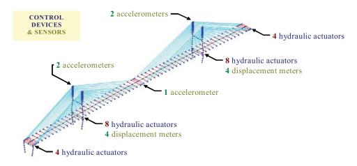
Figure 1. Example of Structural Active Control use [8]
