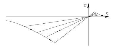
Figure 3: Local damage model with different tension—compression properties.
