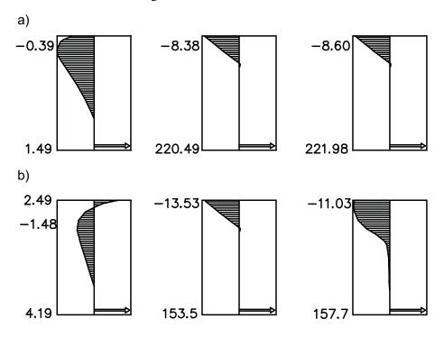
Fig. 6. Stresses in cracked concrete element, concrete B-15 (see Fig.4), steel  $f_y$  = 220 MPa. a)  $\mu$  = 0.5%, M = 29 kNm, b)  $\mu$  = 2%, M = 75 kNm
