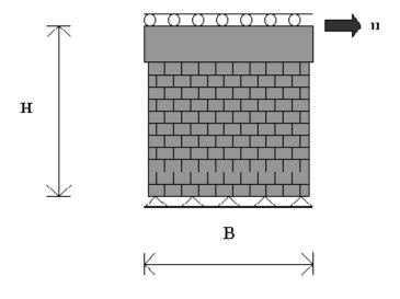
Figure 2. Analyzed masonry panel
