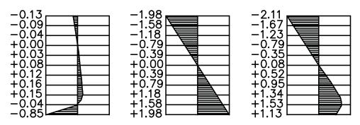
Fig. 4. Results of calculation the self-stress for concrete B-15 ( $f_c$ =15.0 Mpa,  $f_{ct}$ =1.40 Mpa,  $E_c$ =23.1\*10<sup>3</sup>MPa).
