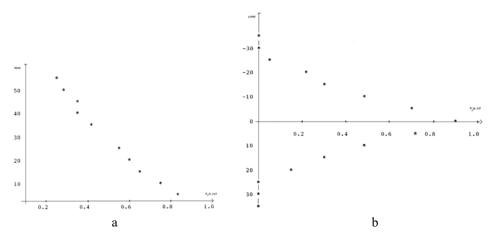
Fig. 5 a, b. Correlations obtained in the boundary layer wind tunnel SECO 2 during the process of modelling the wind turbulent flow ( z=15 cm ): a)- longitudinal correlations; b)-transversal correlations [6]
