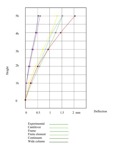
Fig.1. Level Lateral Displacements on Design Models
