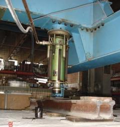
Figure 2. The stand for dynamic testing of bridge models at great scale
