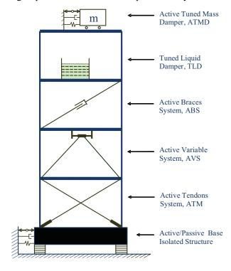
Figure 2. Use of some structural control systems [27]
