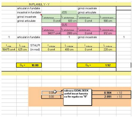
Figure 5. Values of G factors and calculation of the buckling factor
