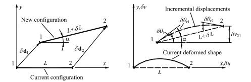
Figure 1. Incremental displacements of the beam
