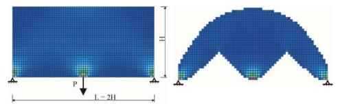
Figure 6. Design domain and ESO solution for R = 5%.
