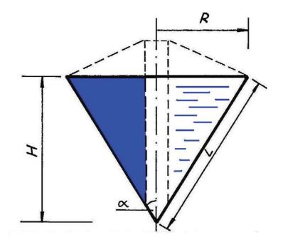
Fig. 2. Steel tank – lump and design variable  $\alpha$
