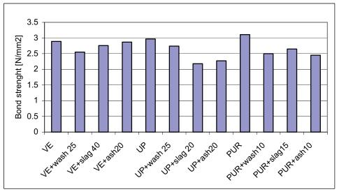
Fifure 3. Bond strength of polymer coatings to concrete surface. VE+wash25 – VE binder filled with 25 % of waste washings. Other abbreviations are analogous
