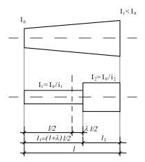
Figure 2. The equivalent beam
