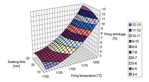
Figure 1. Firing shrinkage – constant pressing pressure 35 MPa.
