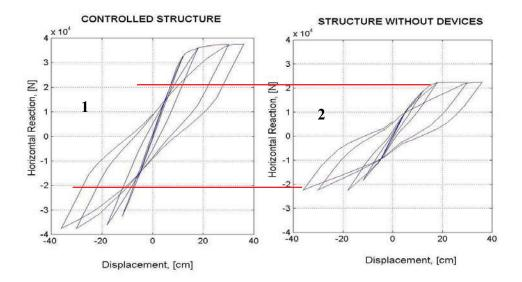
Figure 4: Hysteretic cycles. 1: Structure. 2: Energy dissipating devices.
