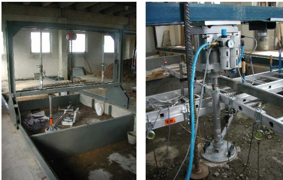
Fig. 1 – Laboratory Geotechnical Testing Field (GLTF) left – general view with static plate test, right – equipment for cyclic loading
