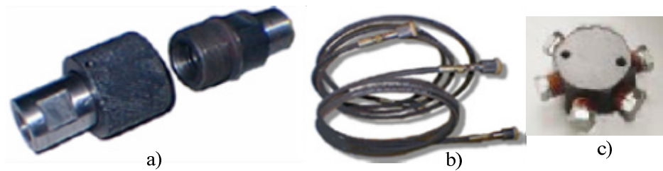
Photo 22. Hydraulic drive unit fittings: a) Quick high voltage coupler; b) hydraulic hose; c) branch hydraulic systems
