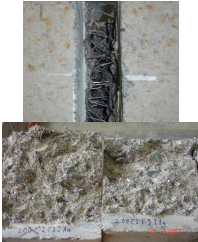
Figure 10 - Fibre pull-out of a cracked SFR-RCC specimen
