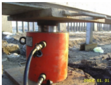
Photo 20. Hydraulic cylinders with double action
