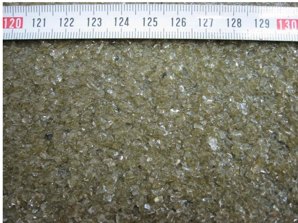
Figure 3. Representative sample where 50 % of fraction 1 - 2 mm was used (on concrete block of thickness 50 mm)
