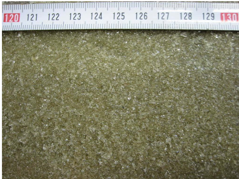
Figure 3. Representative sample where 67 % of fraction 0,25 - 1 mm was used (on concrete block of thickness 50 mm)
