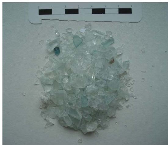
Figure 1. Recycled container glass before the pre-treatment
