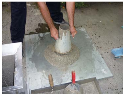
Fig. 3 - The flowing test, made with cone and a non-absorbing plate
