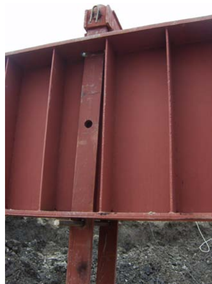
Fig. 2.3.3. Detail thrusts-beam test fixture
