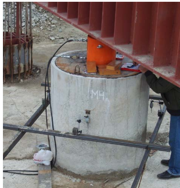
Fig. 2.3.1. Pilot called compression fittings
